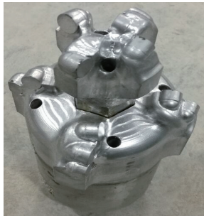
图 5 室内试验专用中心差压式钻头 Fig.5 Special central differential pressure drill bit for laboratory experiment
