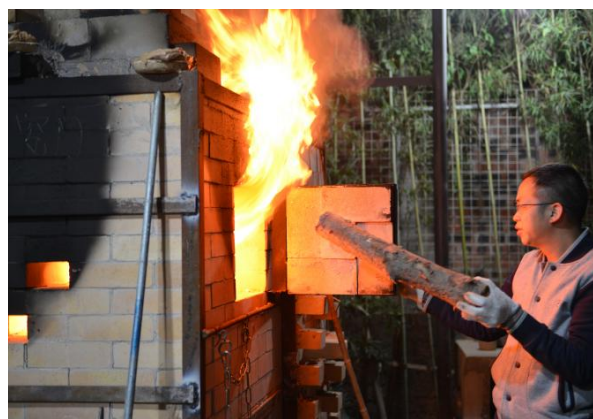
图 8 笔者利用日式高效柴窑烧制作品 Fig. 8 The highly-efficient Japanese-style smokeless wood-fired kiln with the ceramics created by the author
