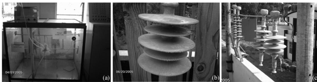
Figure 2 Photographs of aging test facilities developed by University of Engineering & Technology, Taxila, Pakistan. (a) Lab aging chamber with humidity, temperature and other parameters control; (b) insulator installed in a polluted industrial area of Pakistan during hydrophobicity test; (c) polymeric insulators installed in outdoor environment of Pakistan under natural aging tests since last two years.
