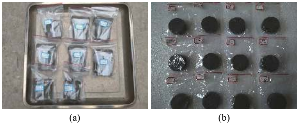
图 2 试样密封养护 Fig. 2 Samples sealed for preservation
