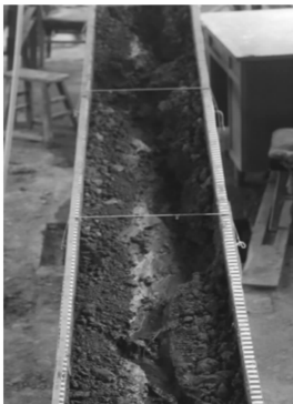
图7 高坡度细沟流道左右摆动 Fig.7 Higher slope condition rill flow swinging
