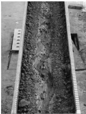
图5 低坡度跌坑数量较少、深度浅 Fig.5 Lower slope condition small,shallow depth of drop pit
