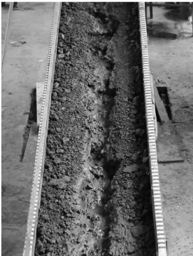
图6 高坡度跌坑数量多、深度加深 Fig.6 Higher slope condition number,deep depth of drop pit
