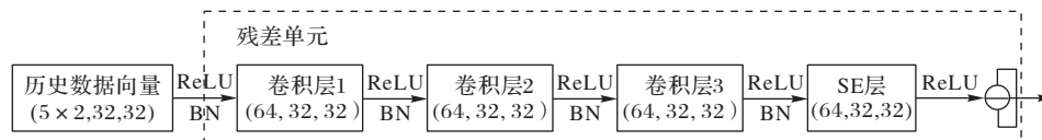
Fig. 3 Residual unit structure of SECLI
