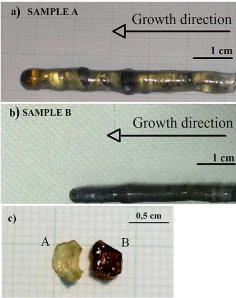
Fig. 1. (a) As-grown single crystal grown in dry air. In this case, there is no dark phase and the sample has a pale yellow color. (b) As-grown single crystal grown in oxygen, showing a dark color. (c) A comparison between a synthesized piece cleaved from a crystal grown in oxygen (on the left) and a piece of crystal grown in dry air (on the right).
