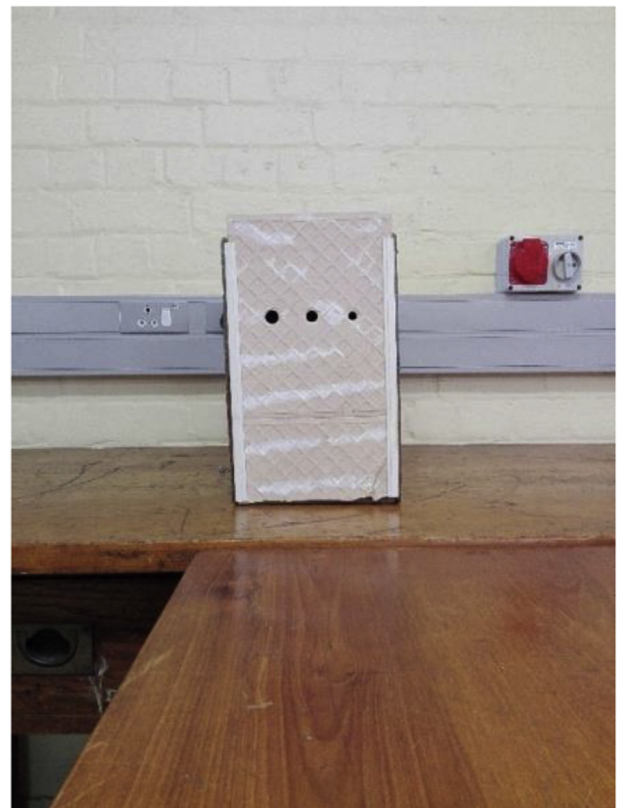
Fig. 5 Optical image of a tile with 16, 14, and 10 mm-diameter holes as an example of the setup.
