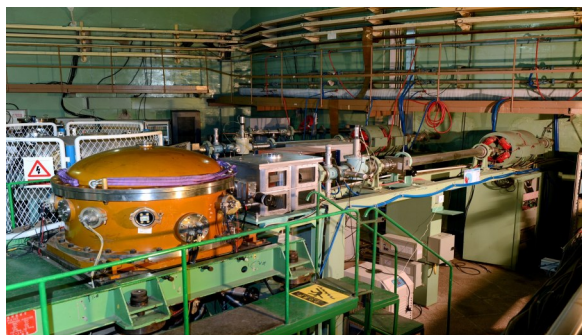
图3 基于北京HI-13串列加速器的重离子微束装置 Fig.3 Heavy ion microbeam equipment based on the Beijing HI-13 tandem accelerator
