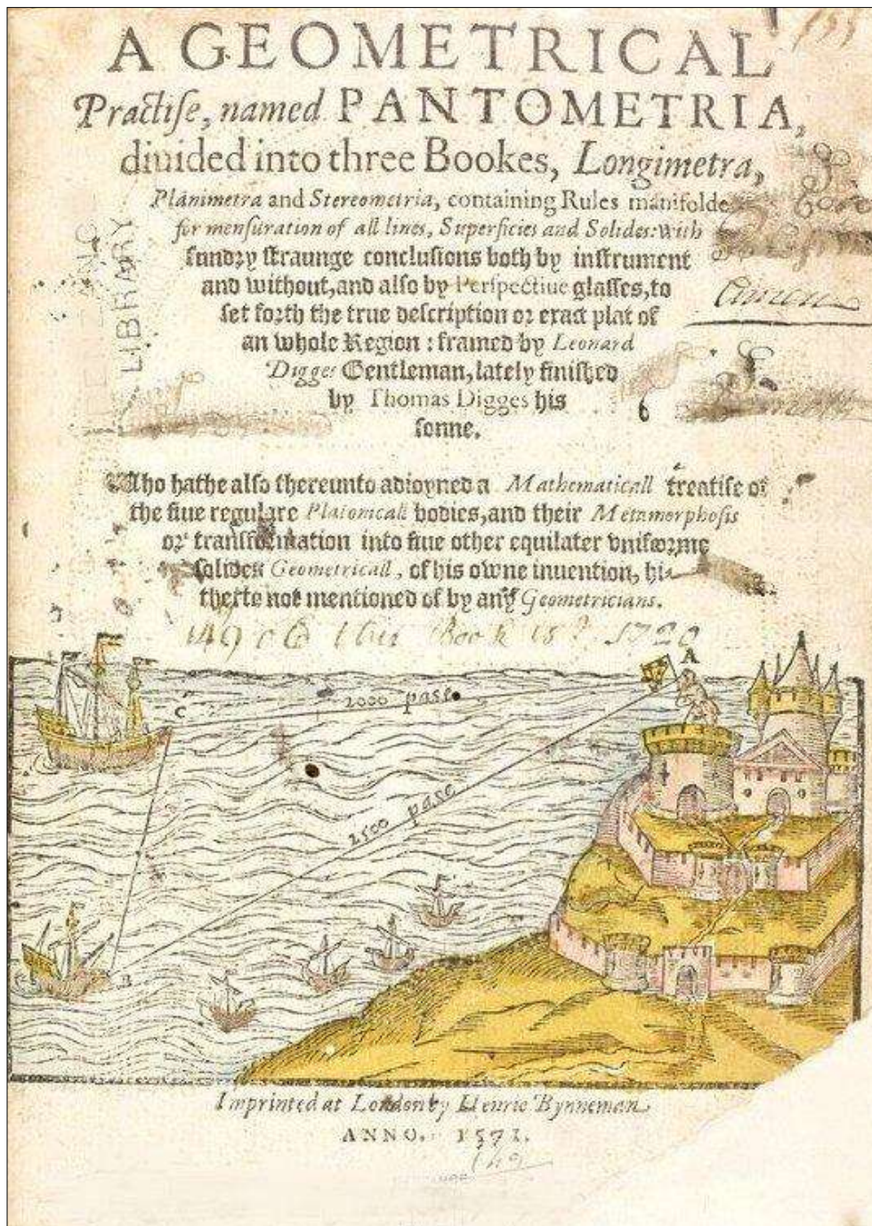
Figure 2: The frontispiece of the edition of 1571 of Pantometria written by Leonard and Thomas Digges, showing some floating ships and an observer on a tower measuring their distances.
