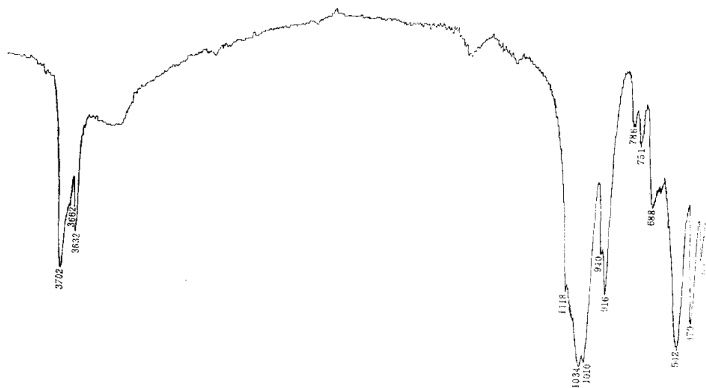
图11-1 紫矸的红外吸收光谱分析 Fig.11-1 IR analysis of the brown kaolinite clay
