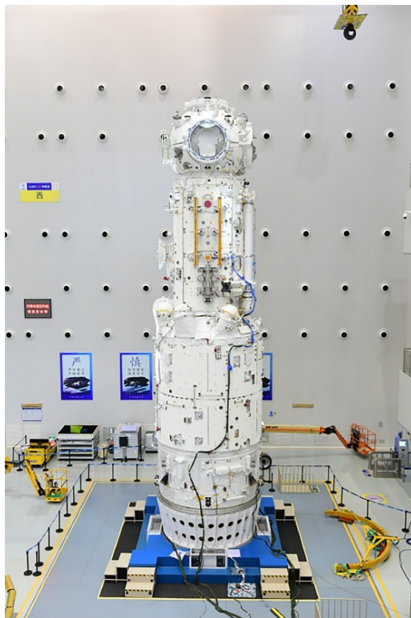
图3 (网络版彩色)天和核心舱整舱振动试验 Figure 3 (Color online) Vibration test of Tianhe core module
