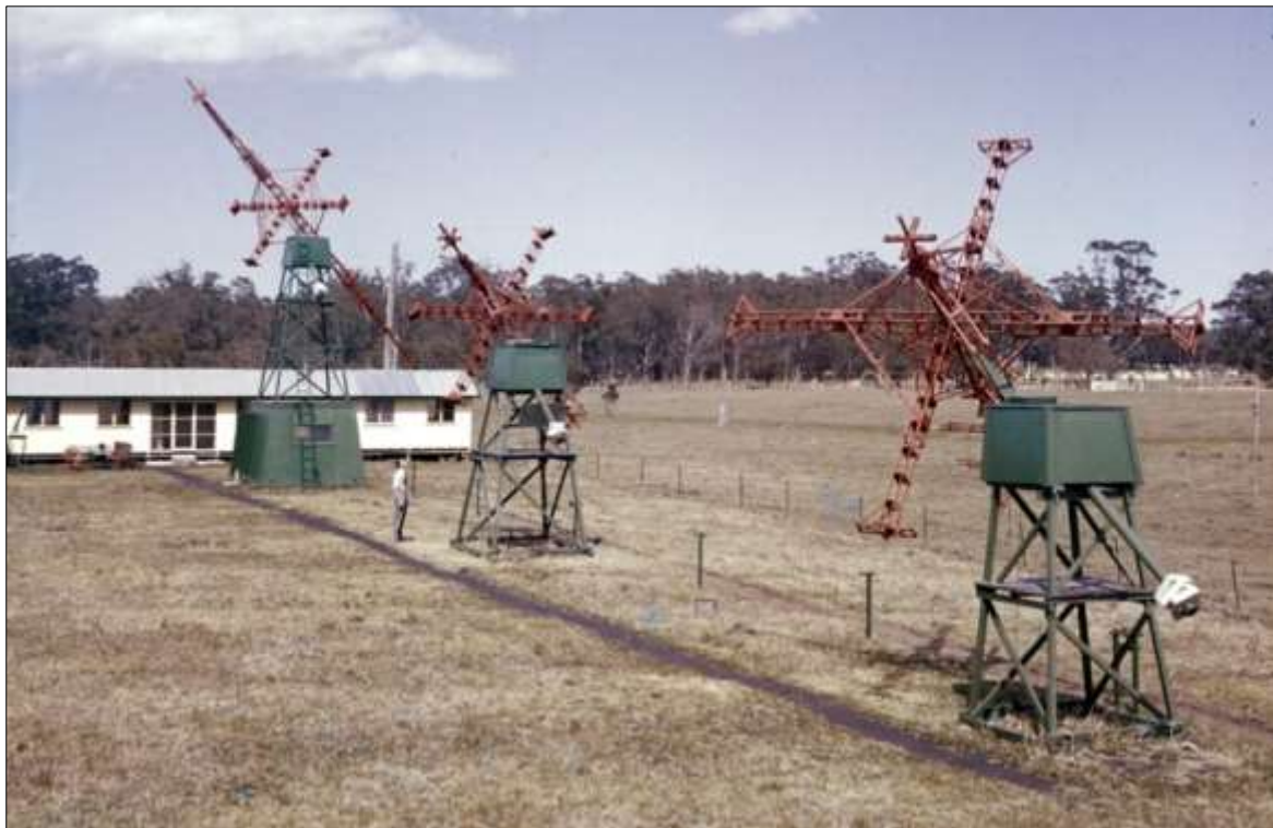
Figure 10: The three original antennas and the receiver building at the Dapto field station. Crossed-rhombic antennas were used so that the polarization of the bursts could be researched (courtesy: RAIA 12429-1).
