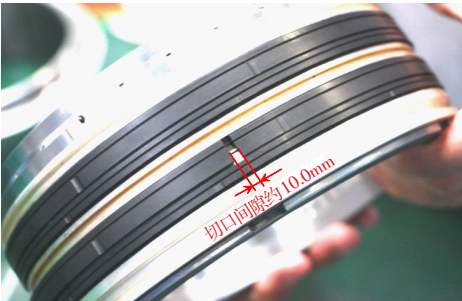
图9 轴间密封环装配后端头弹开形状 Fig.9 Shape of inter-shaft seal ring after installation with deformed end
