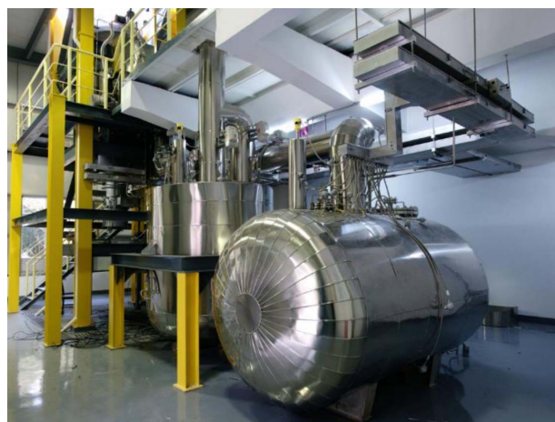
图1 熔盐自然循环实验回路 Fig.1 Molten salt natural circulation experimental loop.
