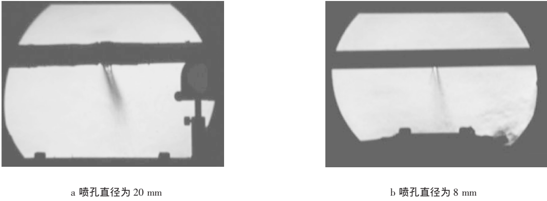
图 6 喷吹压力为 0.4 MPa 时喷孔式喷口气流纹影图 Fig. 6 Schlieren diagram of airflow from jet hole when jet pressure is 0.4 MPa
