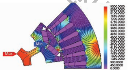
图 13 冻结磁导率条件下的磁力线及相对磁导率分布 Fig. 13 Flux line and relative permeability under frozen permeability
