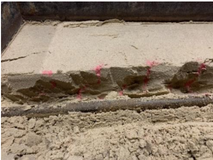
图10 彩砂示踪结果 Fig. 10 Displayed deformational results with color sand
