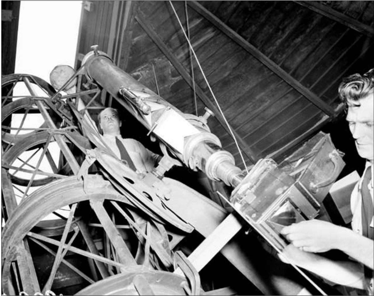
Figure 6: During the 1 November 1948 partial solar eclipse photographs of the Sun were taken with the 6-inch Cooke guidescope attached to the 18-inch Hoskins Telescope at the Central Technical College (courtesy: CSIRO Radio Astronomy Image Archive, B1899-7).
