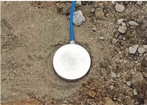
图 1 埋设土压力盒 Fig.1 The placement of soil pressure sensor
