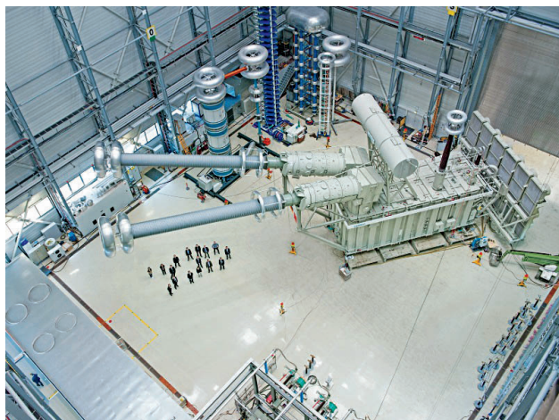
Fig. 4 Prototype test of the 1100 kV bushing at the test bay of the Nuremberg transformer factory
