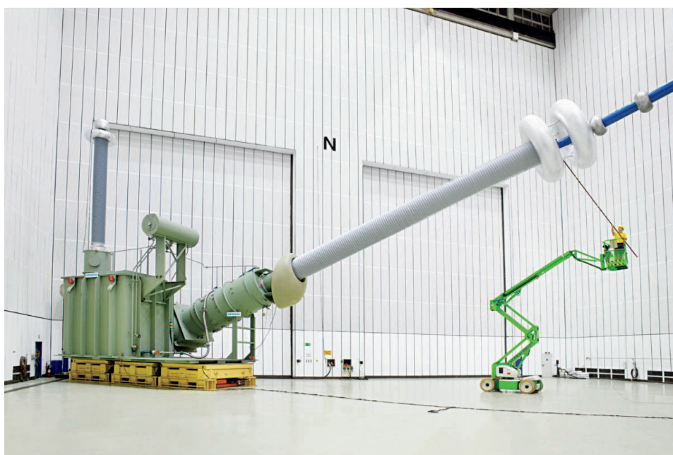
Fig. 3 Prototype test of the 1100 kV bushing at the test bay of the Nuremberg transformer factory
