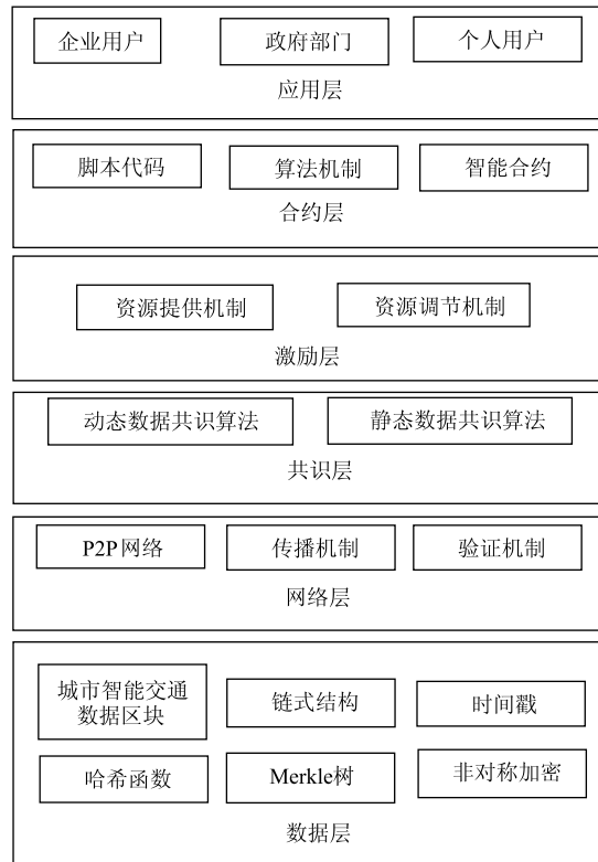
图3 区块链技术的城市智能交通大数据平台的基本架构 Fig.3 Basic architecture of urban intelligent transport big data platform based on blockchain technology
