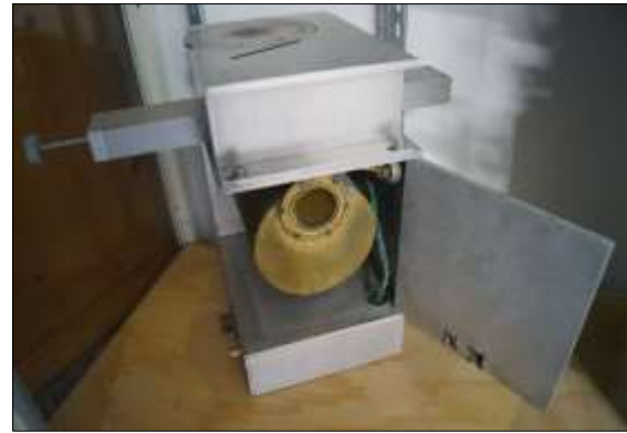
Figure 10: The UBV cold box/1P21 refrigeration box for the single-channel photoelectric photometer. This has been highly cannibalized, but one can still identify the filter bayonet (the horizontal structure), the diaphragm wheel at the very top, and the hole in the bronze cylinder where the PMT (1P21) should be inserted. The bronze cylinder would be filled with crushed dry ice as refrigerant and should be surrounded by silicon dioxide powder (Santocel) as thermal insulation (photograph: W.J. Schuster, 2022).
