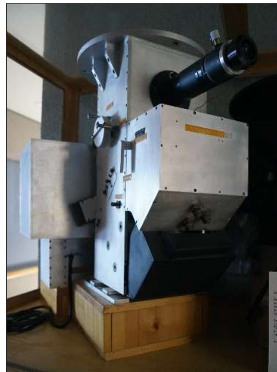
Figure 11: One of the infrared photometers developed by Dr Johnson and his team, left at the Observatory at San Pedro Mártir, and referred to as the ' JHK infrared photometer' (and the ' IJK ' photometer in some of Dr Johnson's letters). It uses the PbS detector 'A' of Dr Johnson. In this photograph the chopper unit is painted black, the standard source module is above this, the detector module is behind the photometer at about the same level, and the electronics (amplifier) module beneath this. Only the very end of the filter bayonet can be seen protruding from between the photometer body and the detector module; the three filters remain installed (photograph: W.J. Schuster, 2022).
