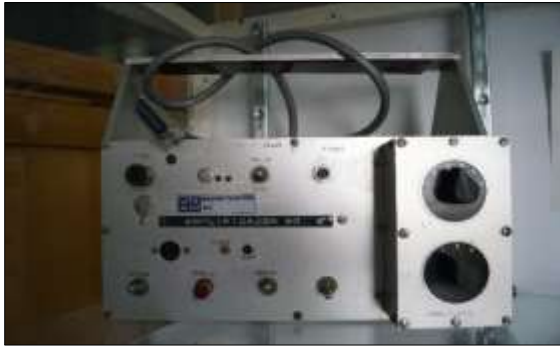
Figure 12: The DC amplifier No. 6, which appears very similar to amplifiers 1 and 4, which were used much more at the Observatory at San Pedro Mártir, but have been highly cannibalized. The 0.5 and 2.5 magnitude gain steps, adjusted by the two knobs on the right, were calibrated every 3–6 months using the apparatus of Ortega (1971) (photograph: W.J. Schuster, 2022).
