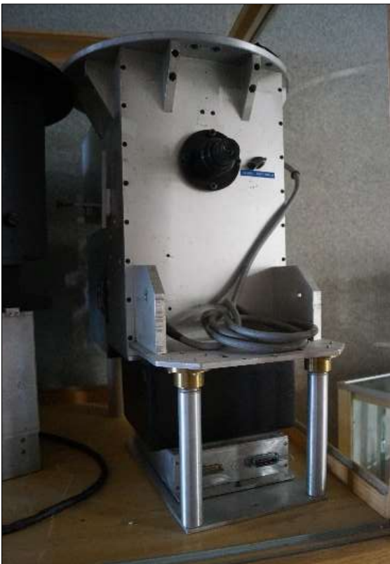
Figure 13: A Johnson photometer found and refurbished by the mechanical technicians of the Institute of Astronomy, Ensenada, for possible use in a site museum, which eventually never included this instrument. The black box is wooden, and has been provided only so that this 'unknown' photometer can be displayed upright with its mounting plate at the top (photograph: W.J. Schuster, 2022).
