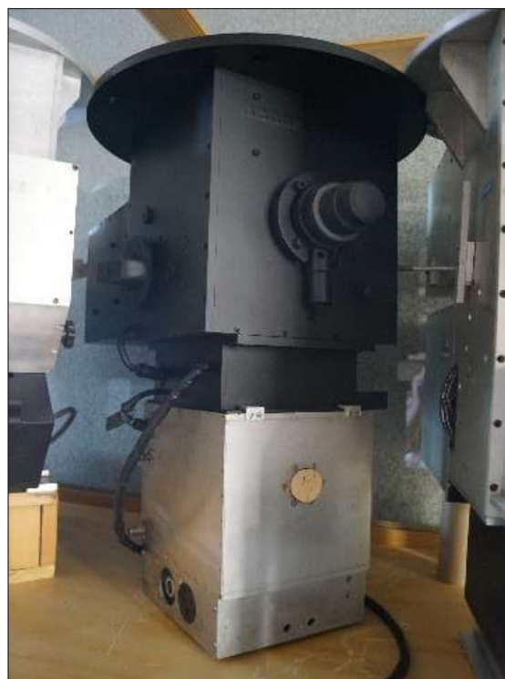
Figure 7: The 8C photometer as seen in its display case in Ensenada. The mounting plate, photometer head, transition module, and cold box can be discerned as well as part of the standard-lamp module at the back. The eyepiece at the front of the photometer head is a simulation plastic replacement, since the original has been lost. The cork stopper at the front of the cold box can be removed to fill the cold box with crushed dry ice for refrigerating the PMT (1P21) (photograph: W.J. Schuster, 2022).
