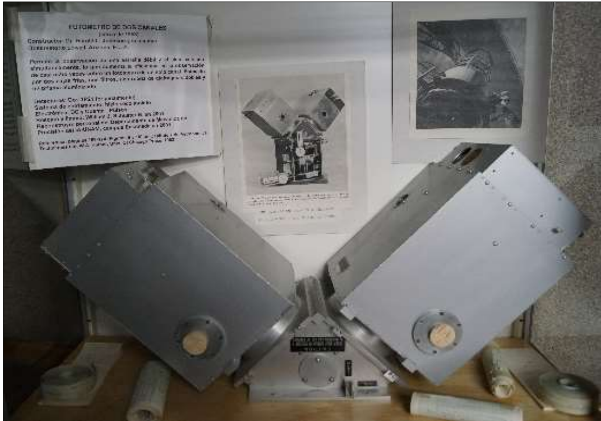
Figure 9: The double photometer as shown in its display case in the Harold L. Johnson Museum in Ensenada. These cold boxes hold RCA 7102 photomultiplier tubes for RI or 6RC photometry rather than the original 1P21s for UVB. The triangular ‘heart’ of this double photometer in the bottom centre of the photograph contains the double-diaphragm disk and the aluminized prism for separating the ‘star’ and ‘sky’ channels; an eyepiece could be introduced for guiding. The two corks show where crushed dry ice can be inserted for cooling the PMTs. The middle photograph in this display case is after Johnson (1962: Figure 10) , and the right-hand photograph shows this photometer being used with the 74-in telescope of the University of Toronto. The rolls and strips of paper at the bottom of this display case indicate how the photometric data from the first years at the San Pedro Mártir Observatory were frequently taken and reduced: printers and chart recorders, followed by punched paper tape for input into a Nova computer (photograph: W.J. Schuster, 2022).
