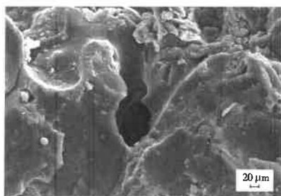
图8 烧结25 min时RSC的SEM图像 Fig.8 SEM image of RSC at calcination time of 25 min
