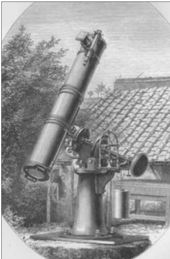
Figure 36: The equatorially mounted 9-inch Newtonian reflector that Pogson used to observe the 1872 annular eclipse (after Tennant, 1869: 51 ).
