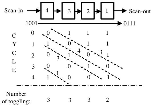
Figure 1 Transitions on scan chain caused by test stimuli and responses.
