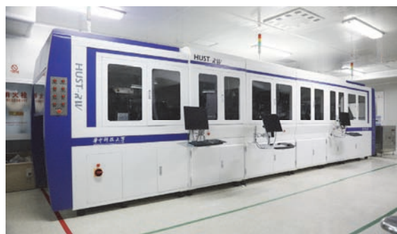
图4 (网络版彩色) 柔性RFID标签卷到卷倒装键合装备 Figure 4 (Color online) R2R flip chip equipment for flexible RFID tags manufacturing
