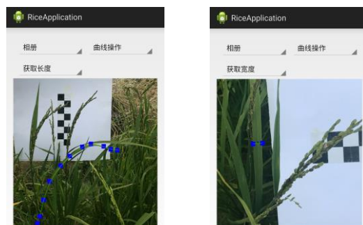
(a)叶长方向3次B样条曲线;(b)叶宽方向1次B样条曲线 (a)Cubic B-spline Curve of Leaf Length Direction; (b)First-order B-spline curve of blade width direction
