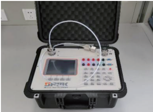
图 4 压力校验仪实物图 Fig. 4 Physical drawing of a pressure calibrator
