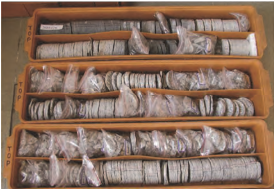
图3 (网络版彩色)CCSD-1井3478~3524 m井段的岩心片化现象 Figure 3 (Color online) Discsed cores obtained in 3478~3524 m section of CCSD-1 well
