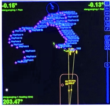
Fig. 4. Walking path ‘SJ’ measured by super-short baseline at 1305 m depth.
