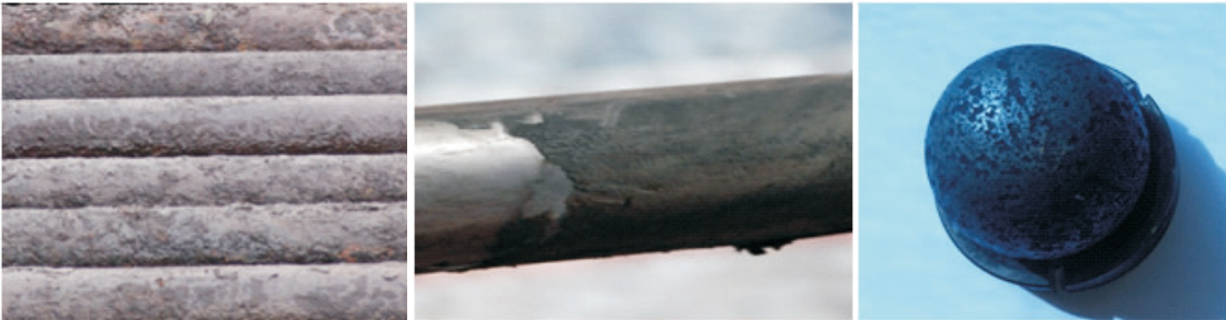
图 1 单井注气三采井油管和泵的结垢腐蚀 Fig.1 Scaling and corrosion of strings and pumps in the third round of oil recovery in gas injection wells
