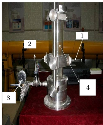
1. Tungsten electrodes; 2. Electromagnetic valve; 3. Pressure gauge; 4. Quartz glass tube
