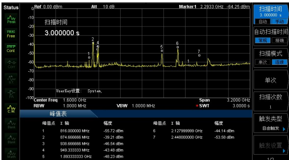
图 4 高架站台频谱仪测量数据 Fig.4 Measurement data of spectrum analyzer on the elevated platform
