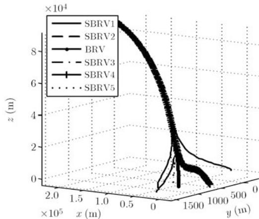
**Figure 2** Three-dimensional trajectories of an invariable-structure SBRV.
