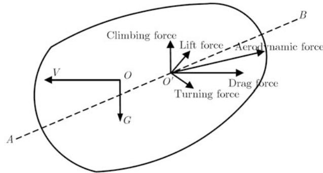
Figure 1 SBRV and geometry of forces.
