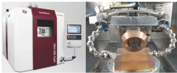
图 10 Optotech UPG 500 CNC超精密磨床磨削过程 Figure 10 Grinding process of Optotech UPG 500 CNC ultra precision grinder.
