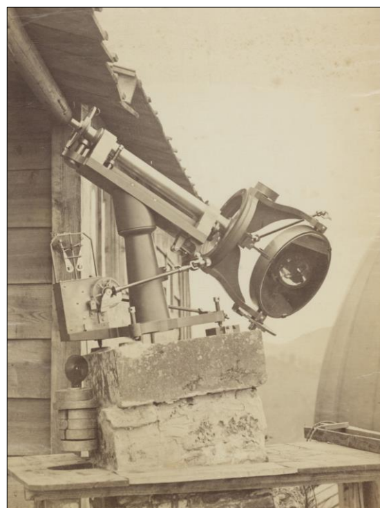
Figure 5: The polar siderostat, for solar observations. The flat mirror has a diameter of 30 cm. It was built for the latitude of Japan where the 1874 Venus transit was observed (courtesy: Paris Observatory Library).
