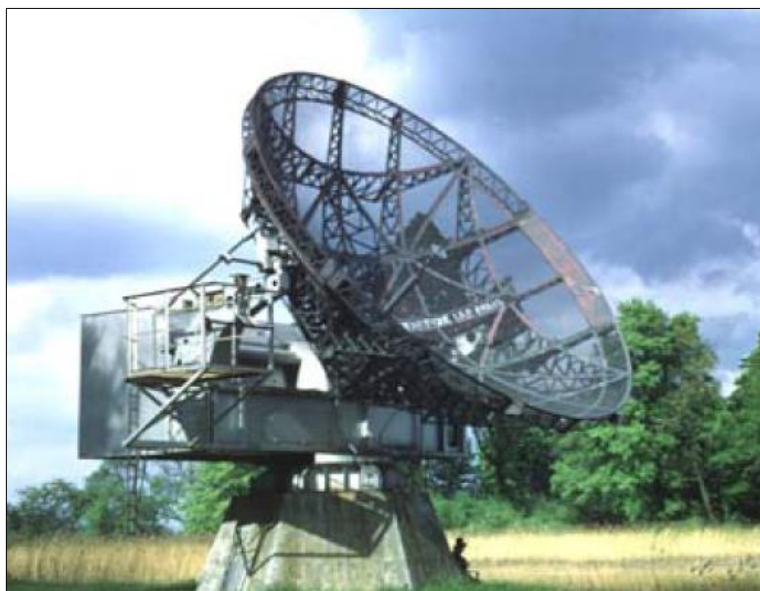
Figure 18: The 7.5-m diameter Würzburg antenna in Meudon, installed in 1947. It was moved in 1962 to the Bordeaux Observatory, but the concrete basement is still visible (courtesy: Paris Observatory).
