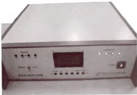
图 5 触发脉冲延时分配器 Fig.5 The trigger pulse delay and assignment apparatus.
