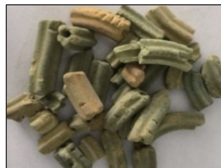
图 1 失活硫酸催化剂样品外观形貌 Fig. 1 Sample appearance of deactivated sulfuric acid catalyst
