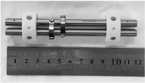
图 2 小型四极杆加工实物照片 Fig. 2 Photograph of manufactured miniature quadrupole mass analyzer
