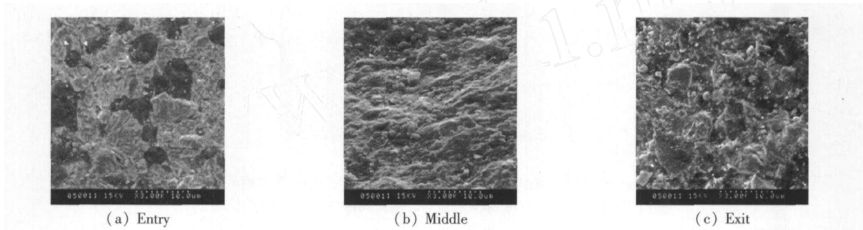
Fig 4 SEM micrographs of the worn bore surfaces of the GN gradient nozzle (after 540 min operation) 图 4 梯度陶瓷喷嘴冲蚀磨损内表面形貌 SEM 照片 (冲蚀 540 min)
