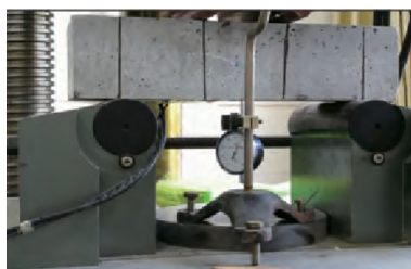
图 2 四点弯曲试验装置和试件尺寸 mm Fig. 2 Four-point bending test device and specimen size
